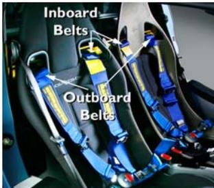
**Note: Please read Schroth guidelines for installing ASM shoulder harness. It is critical that the ASM belt is on the inboard shoulder. The ASM belt has a bright yellow tag sewn in (as shown in the image). The Sector111 Harness Kit is designed to help you install the lap belts on ANY Schroth Profi-II belt system (ASM, HANS, etc).**
