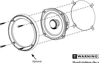
Hand-tighten the screws evenly in a criss-cross pattern to avoid bending the speaker frame or stripping the mounting clips.
