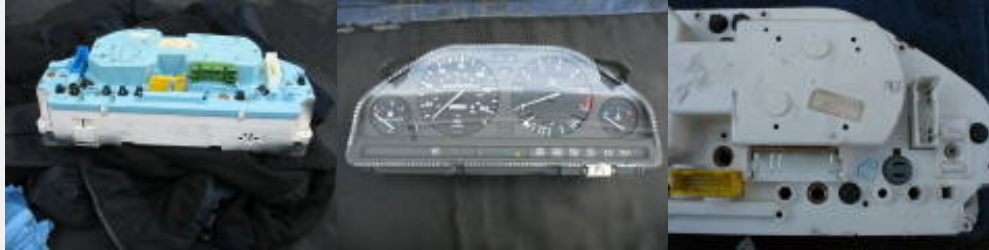
From left to right, the back of a CPT cluster, the front of a CPT (note the coding plug in the lower right of the cluster) and the back half of a NCPT cluster.
