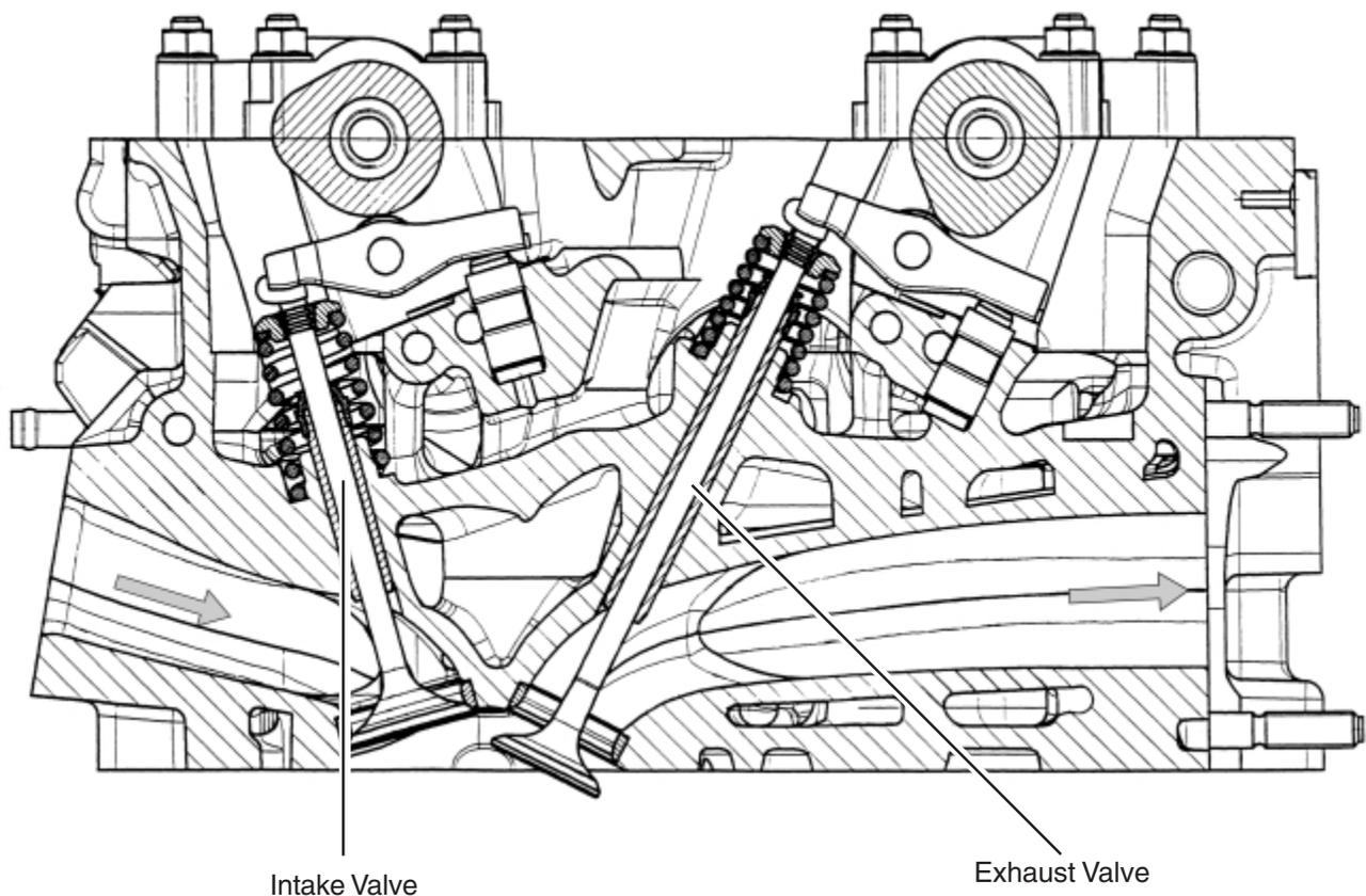
**Cylinder Head Cross-Section View, Cylinders 2, 4, and 6**
