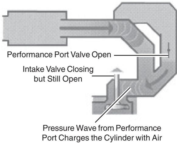
The performance port pressure wave is reflected back toward the intake valve ports, and that air is forced into the combustion chamber before the intake valves close.
