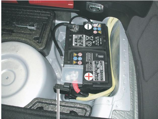
Fuse S138 Connected to Positive Terminal of Battery in Trunk
