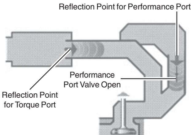
Because the distance it must travel is shorter, the intake wave reaches the open end of the intake duct at the performance port before it reaches the open end of the intake duct at the torque port.
