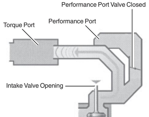
The open end of the intake duct at the torque port has the same effect on the intake wave as a solid wall has on a ball. The wave is reflected back toward the intake valve ports in the form of a high pressure wave.
