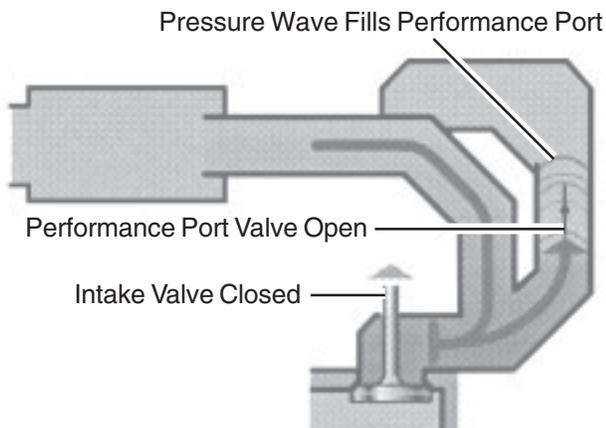
The pressure wave arriving too late from the torque port is reflected by the closed intake valves and pushes its air charge up the intake duct, filling the performance port in preparation for the next cycle.
