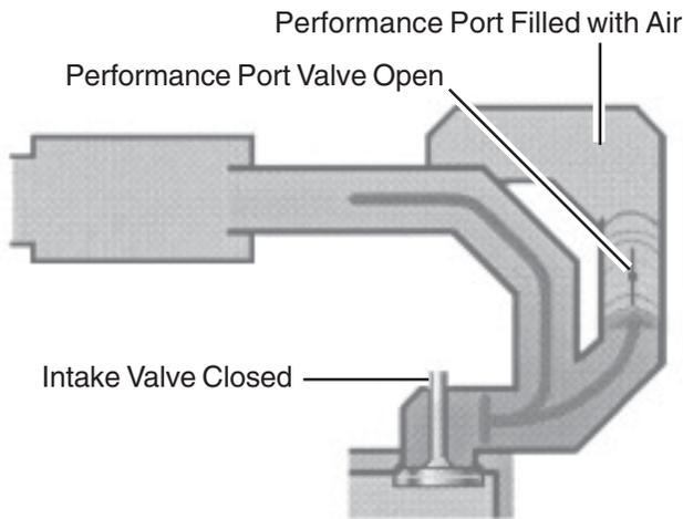
In the 3.2-liter V6 engine, the performance port valve turns to the performance position at engine speeds below 900 rpm and above 4100 rpm. This opens up the path to the performance port. The performance port is designed so that the intake and pressure waves will have a shorter path back to the intake valve ports.
