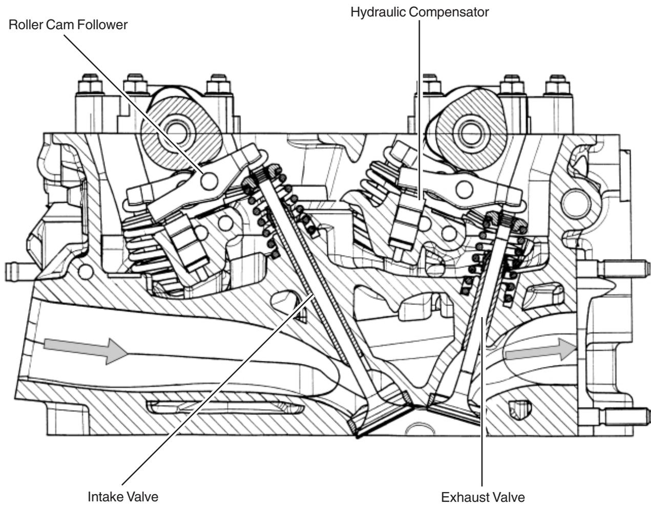
**Cylinder Head Cross-Section View, Cylinders 1, 3, and 5**
