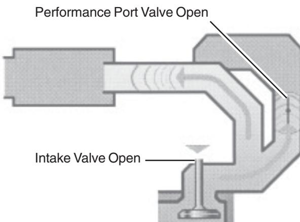
When the intake valves open, the intake wave moves up both manifold intake ducts toward the torque port and the performance port at the same speed.
