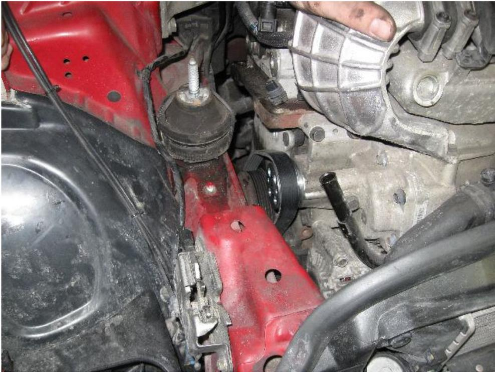
11. Put the belt tensioner back. When the belt tensioner works you can try to screw down 4 bolts of the pulley (because you can not hold the pulley with your hand as much as the belt tensioner).
