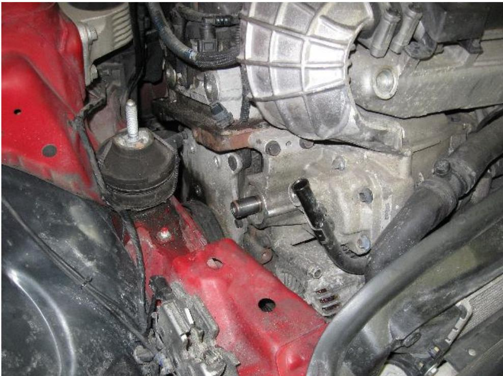
9. Mount the inside piece of the KMT pulley. If it is very tight you can use some sandpaper (1200) on the inside. Put it as back as you can on the shaft. Take the outside piece of the pulley and 4 bolts. Use loctite on them. Hold the outside piece of the pulley to the shaft and screw down the bolts. Tight them as much as you can hold the pulley.
