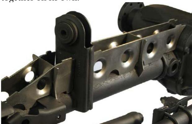
STEP 3. Using a marker or paint pen, indicate the areas on the axle where the truss touches the axle to prepare for welding. Remove truss pieces from axle. Using an angle grinder with either a flapper disc or wire wheel brush, clean the surface of the axle tube, casting, upper control arm mount, and coil perch until bare steel is exposed. Clean surfaces on drivers side casting, tube, and coil perch in a similar fashion.
