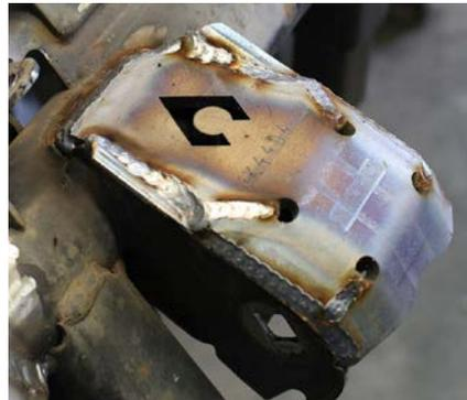
If using a bolt-on raised tracbar bracket that uses a U-bolt, trim piece 4 on the line as shown here.
