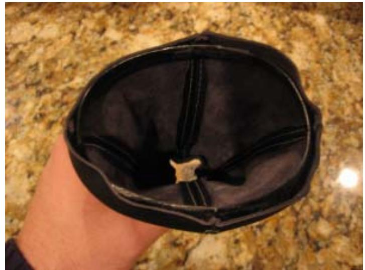
After the glue is dry, the boot can be reinstalled. I started by turning the boot inside out and placing it over the shifter rod. I then zip tied the boot to the shifter rod, be careful to position it so that the reverse cable remains free and functional:
