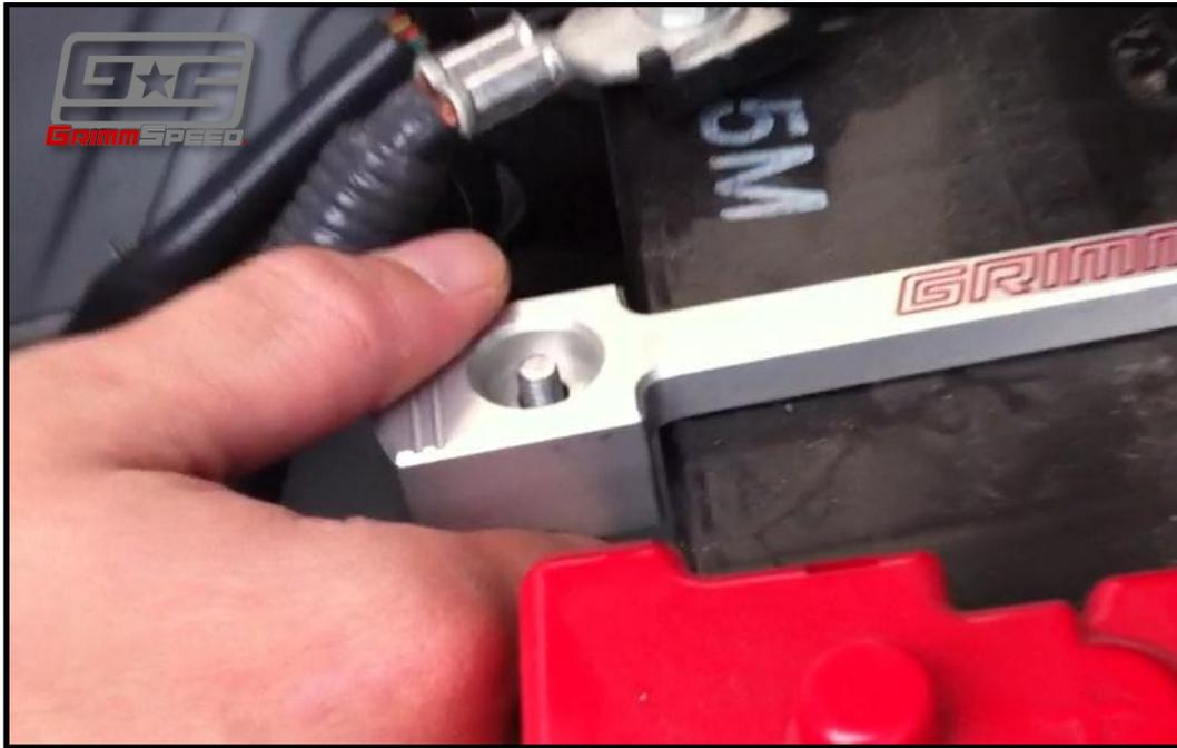
**Figure 3: Hook the front j-bolt.**
