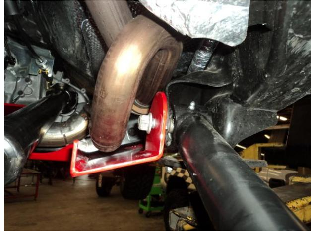
1. Remove factory transference skid (4 bolts: 2 on the center of the transmission cross member, 1 on gas tank, 1 on driver side frame)
