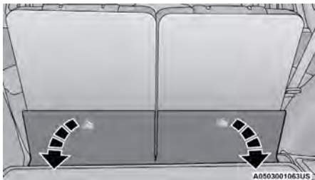
Pulling Down The Carpet Floor Panel To Access Top Tether Anchorage (3rd Row Bench)
