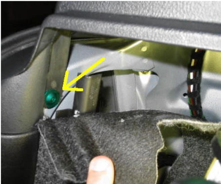
5. Pull back the carpet enough to access the seat belt housing. Make sure to pull the seat belt and wrap it on the seat back of the rear seat. This tension will be useful later.
