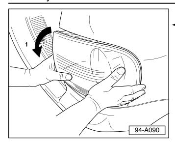
Turn tail light in direction of -arrow- towards outboard side of vehicle until upper edge of tail light housing becomes visible.
