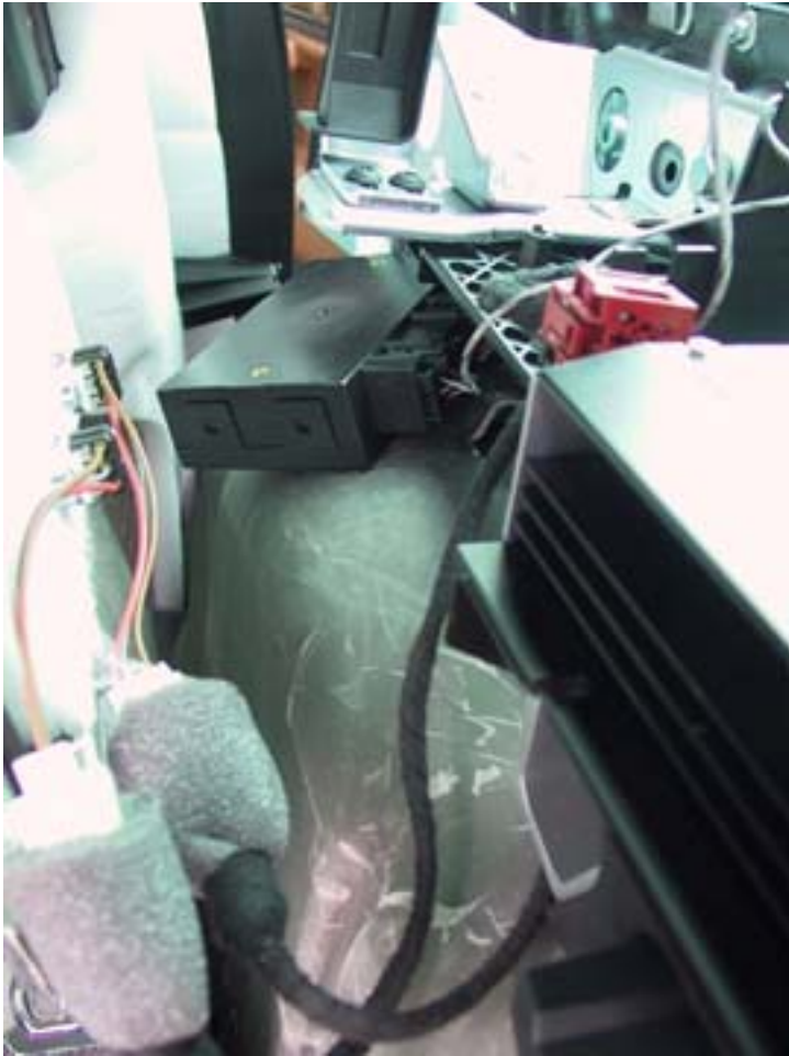
fig 2 Screws removed and module swung out and forward, revealing the rearmost plug. Note the gray wire plugged into the pin #10 socket. NOTE: This is NOT the upper left corner socket, which has a number 9 next to it!
