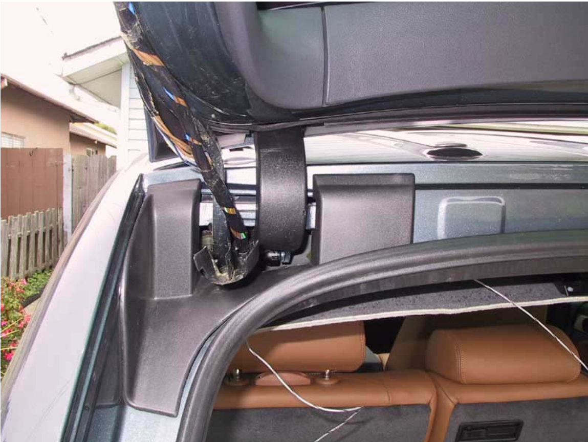
fig 6 Wire harnesses exposed
