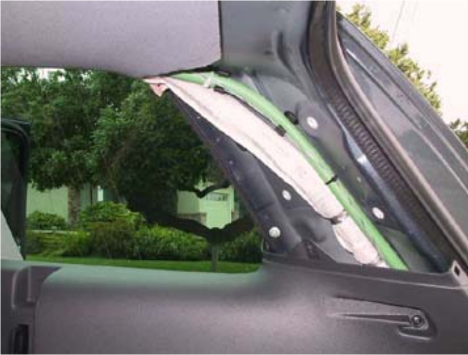
fig 3 Panel reassembled, and wire routed up the D pillar and onto the headliner
