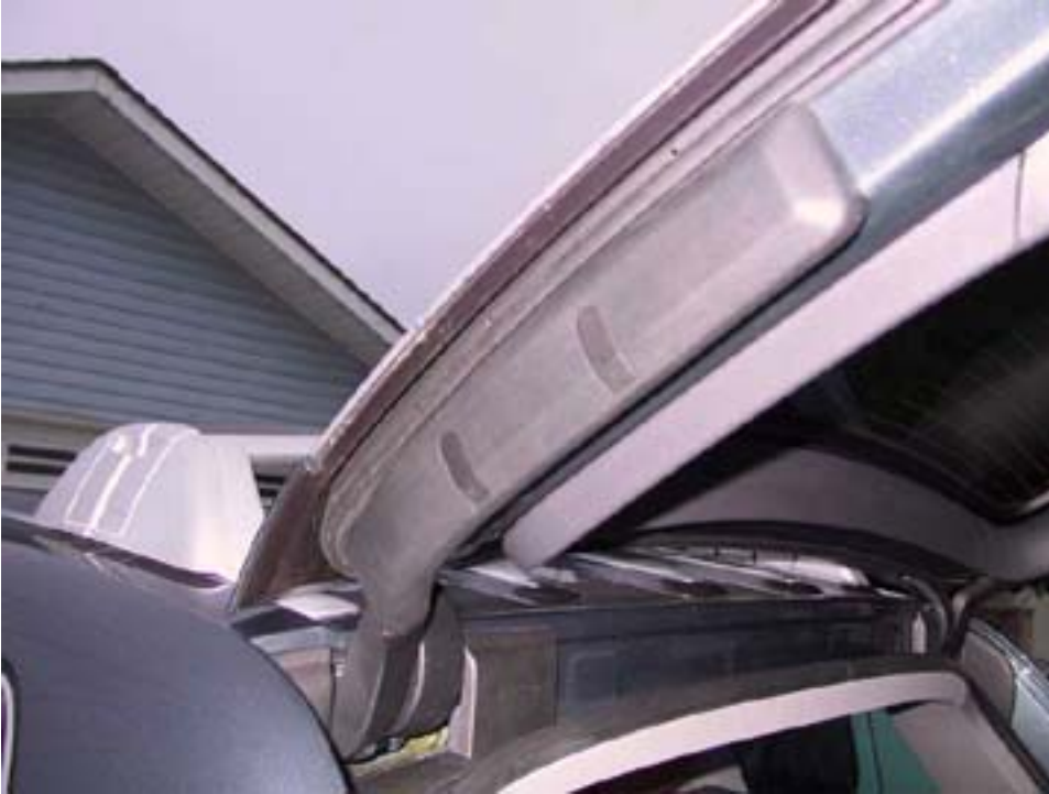
fig 5 Slide the plugs toward their square end, to expose the screws
