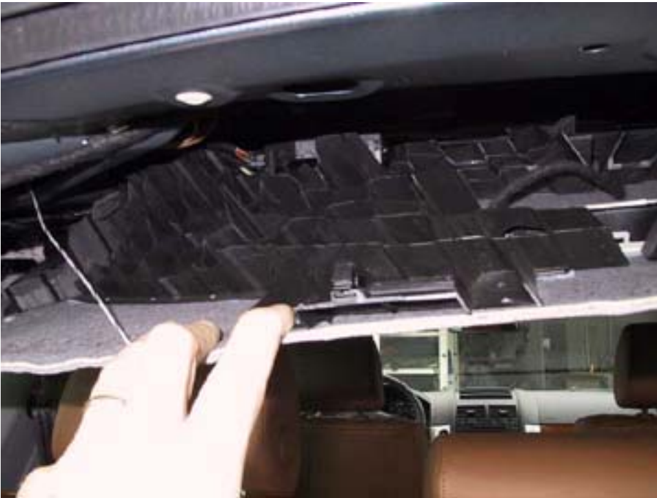
fig 4 Wire runs across the headliner, and forward toward the grommet
