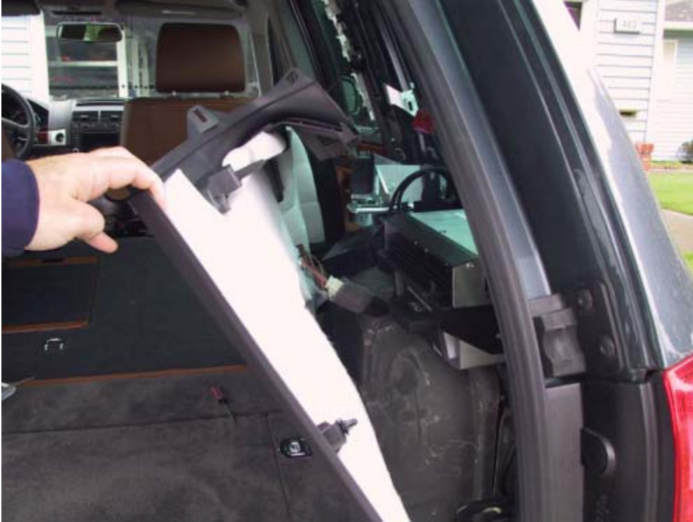
fig 1 Panel released and swung open.
