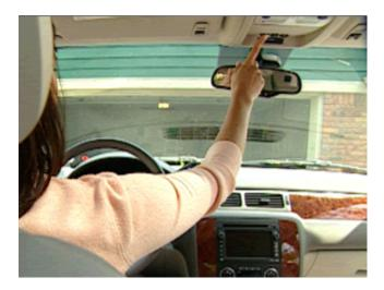
Immediately (within 1 second) release the button once the garage door moves. During this time the selected button indicator light will blink slowly. Do not release the button until you see the garage door move. Most garage doors open quickly. You may need to hold the button from 5-55 seconds before observing movement of the garage door.
