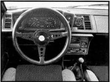
Scirocco's newfound speed and grip. Inside, a classic three-spoke, leather-wrapped steering wheel directs these components. A boost gauge, mounted in a beautifully executed housing to the right of the instrument binnacle, monitors the engine's efforts. The only other interior change is special Callaway-emblazoned upholstery fitted to the otherwise stock seats.
