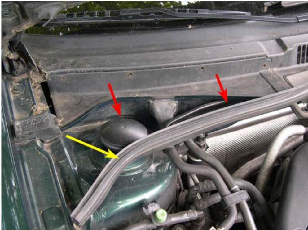
4. After pulling the cover part way out, you'll need to lift it up slightly to allow two wide tabs on the bottom of the cover (indicated by the arrows in the picture below) to clear the lip at the front of the plenum.
