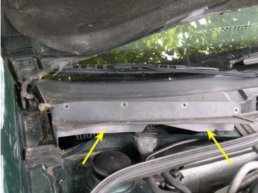
5. With the pollen filter plenum cover completely out, it is easy to see the pollen filter (indicated by the arrow in the picture below) seated at the top of the blower motor assembly.
