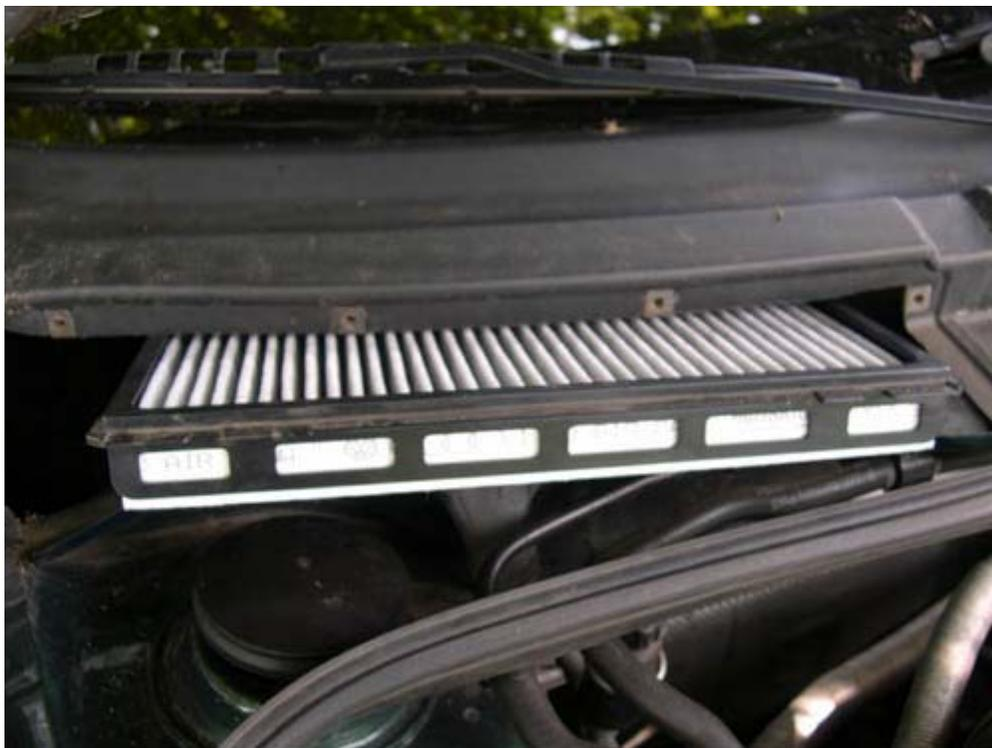
12. The picture below shows the filter frame and filter correctly reinstalled. If the reinstallation is done correctly, the two retaining tabs on the front edge of the frame should click into place easily and there should be no gaps between the filter frame and the top of the blower motor assembly on the sides. It's hard to describe, but you'll be able to tell when the frame and filter are installed correctly.
