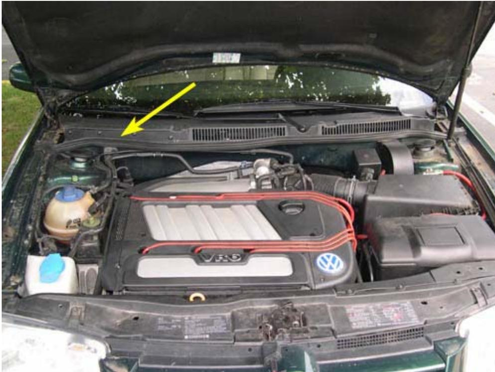
2. Remove the four T25 Torx screws from pollen filter plenum cover. These screws are indicated by arrows in the picture below.
