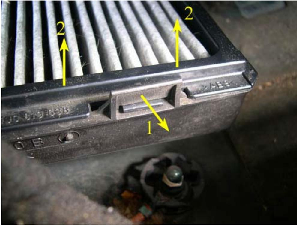
7. The picture below gives a better view of how much pollen and debris the filter actually prevents from getting into the cabin of the car. While the filter in the picture had not been changed in about 50k miles, I routinely scraped the pollen and debris out from between the fins. The space between the fins was free of pollen and debris only 4k miles before these pictures were taken.
