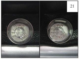
**Bolt on left:** Properly tightened; lower edge of inner piece runs straight
