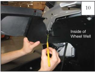
Mark the front portion of the splash shield with a grease pencil in location shown in preparation for trimming. The splash shield should be flush with the sheet metal after being trimmed. NOTE: If trimmed too little, flare won't fit; if trimmed to much, shield won't stay behind flare.
