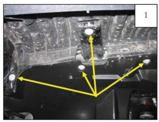
Using a socket wrench with a 10mm socket, remove four factory bolts from inside of splash shield. Save bolts for reinstallation.
