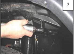
Using a socket wrench with a 10mm socket, remove one bolt located in hole inside of splash shield.
