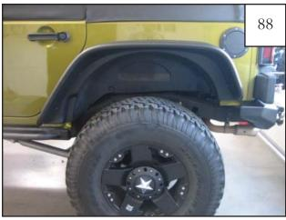
Completed rear driver's side flare installation.
