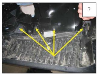
Use a pry tool or flat head screwdriver to remove four plastic fasteners.
