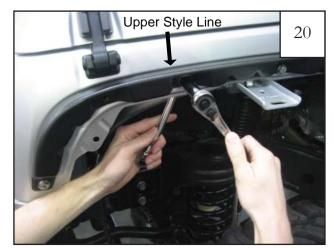
**Step 4** Using a 1/2" socket wrench and a 1/2" wrench, tighten all bolts until inner piece is snug against fender and washers do not spin. *Do not overtighten:* see step 21. Inner piece should rest along upper style line of sheet metal radius and not below it: see step 22.
