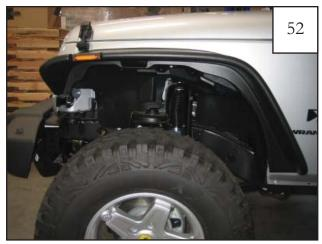
Completed front driver's side flare installation.
