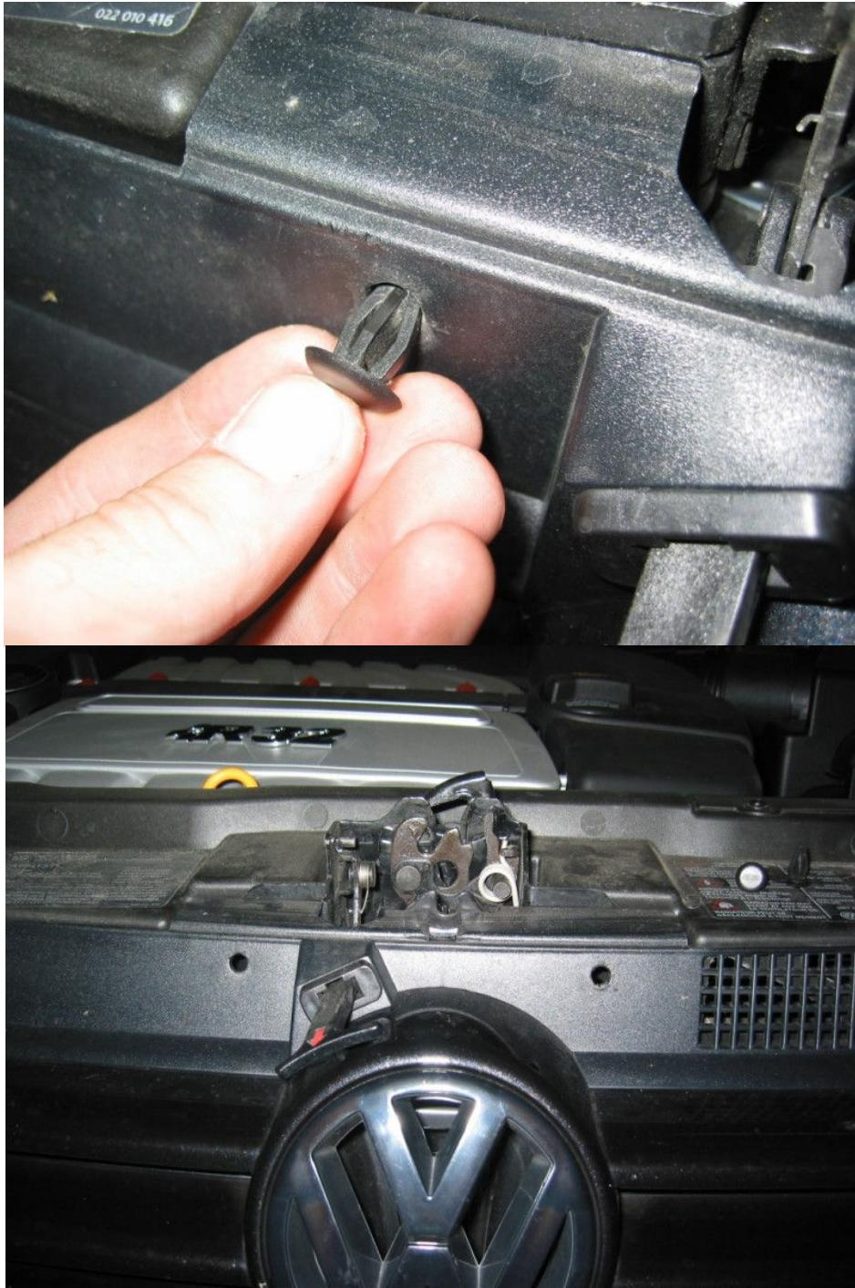
Step 2 – Insert screw driver here, unlock grille:
