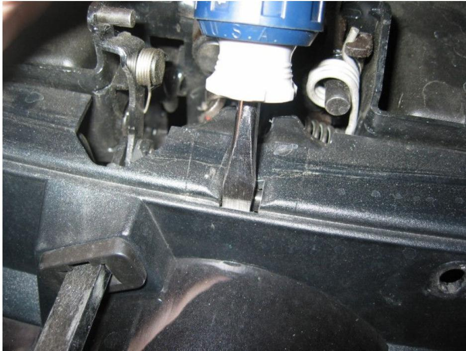
Step 3 - Grille pops up out of the plugs on the bottom of it. The way it detaches from the hood latch is kind of weird, you pull up on a metal tab to unlock it, then stick a screw driver in between the two "fingers" and turn it to pull them apart. You'll see.
