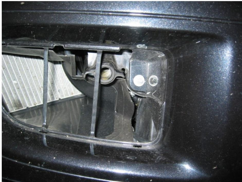
Step 7 - With the nuts removed, the bumper should be able to pull slightly forward to expose the lower bolts: (only pull one side forward at a time so you don't have to pull the whole bumper off)
