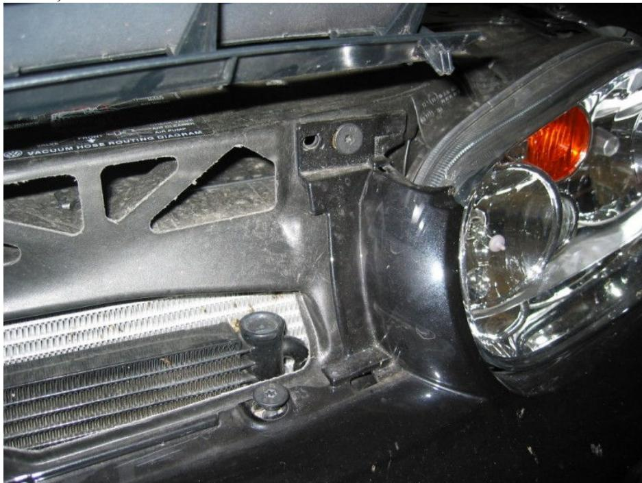
Step 5 - Remove these torx bolts (same size as above) as well as the ones on the bottom front of the bumper that attaches the plate to it:
