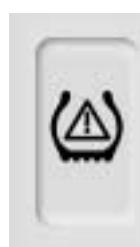
Set or calibration button, most often in the area of the center console or in the dashboard at the right beside the steering wheel.
