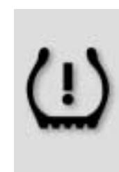
TSS symbol on the instrument panel (lights up when ignition is switched on).
