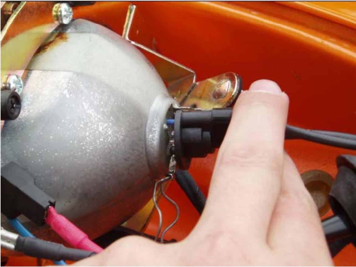
With LOTS of manipulation of the clips, using your needle nose pliers, get them to clip back down under the metal tab. I found it easier to bend the metal tab about 30 degrees out to fit the metal clips under. The metal tab was where the OEM negative wire connected.
