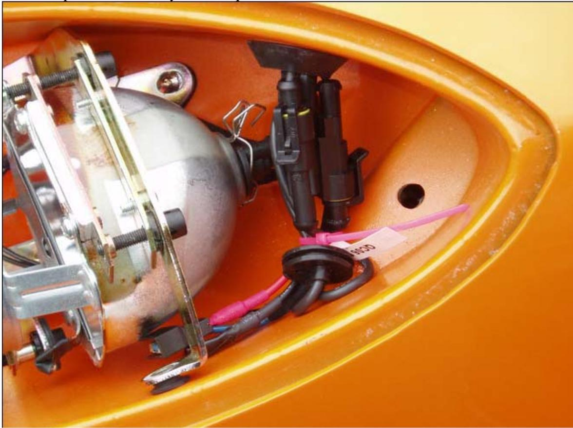
Back underneath you need to use more fancy colored quick ties to wrap all that excess wire up. You notice that I have already re-mounted the light assembly (the nuts are back on),
