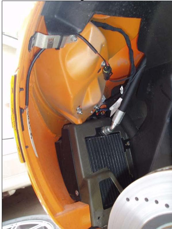
A close-up of the area you will be working on. The three nuts hold the lamp assembly to the clam. The three alen-bolts hold the lens cover to the clam.
