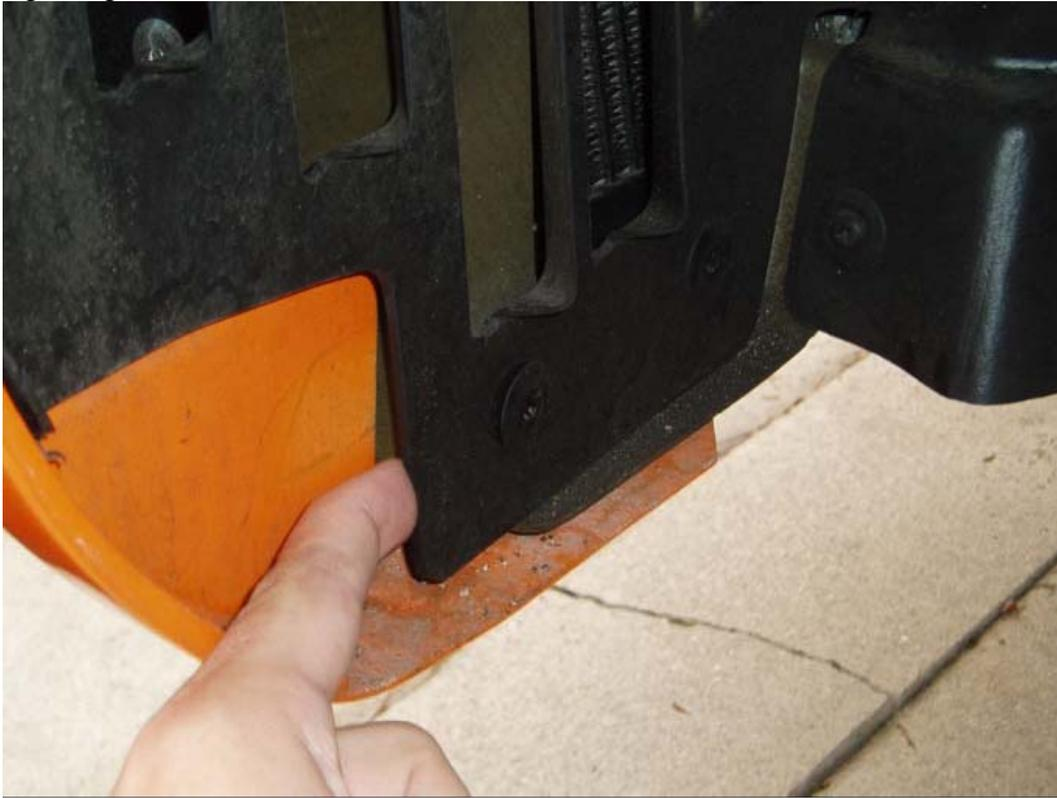
At the top of the plastic guard it slides into the adjacent piece, this is why you remove in a downward motion.
