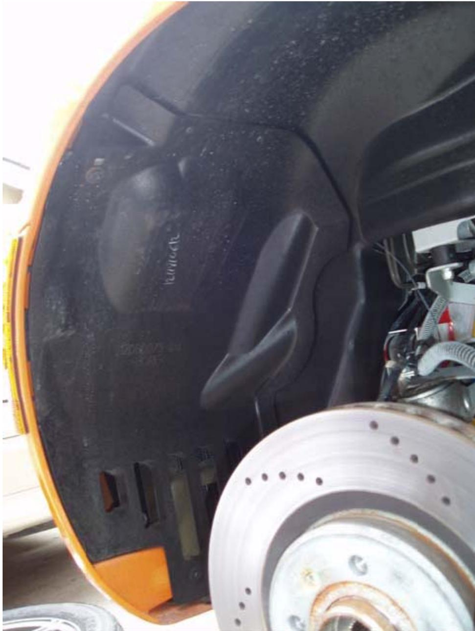
The two on the bottom are the plastic type that don't really screw into anything other than their plastic bases that then expand in their hole.
