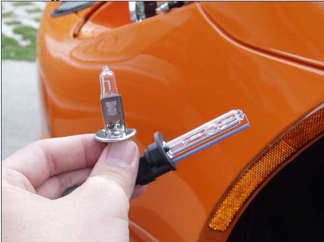
You will notice that the base of the new bulb has a flat side to it. This is important to note. Also there are two 'bumps' that rise out, shown at 1-o'clock and 8-o'clock in the picture. These 'bumps' sit into holes in the light housing assembly so that you make sure you get that bulb in correctly. The flat side allows for clearance from the OEM negative male connector. If they don't go into the holes, or it looks awkward you have done something wrong.
