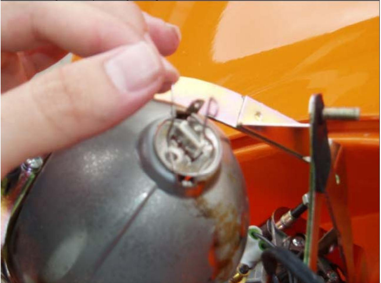
Take the new bulb out of the protector, and remove all that housing stuff. You should have JUST a bulb and the pair of wires coming out of it that run through a rubber washer, NO plastic washers/caps or foam.
