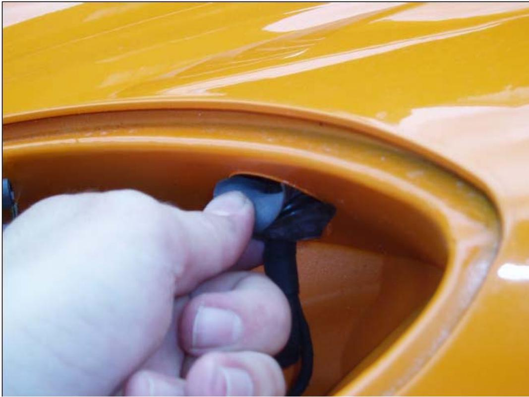
Now assemble the wires that connect to the ballast. The two male ends (3-o'clock in the picture below) are going to plug into the female ends that originally plugged into the back of the OEM light bulb (shown prior). The middle connector/adaptor gives us some length. The ballast is not shown here (sorry), but just off to the right. The plug assemblies are designed to only allow you to construct this in one manner.
