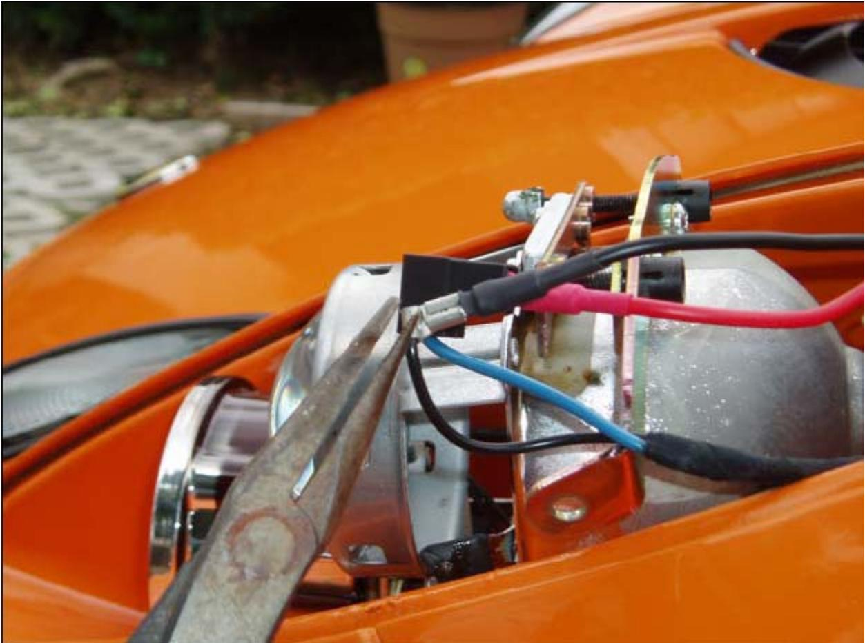
Now pull out the OEM light bulb by undoing the clips as shown.
