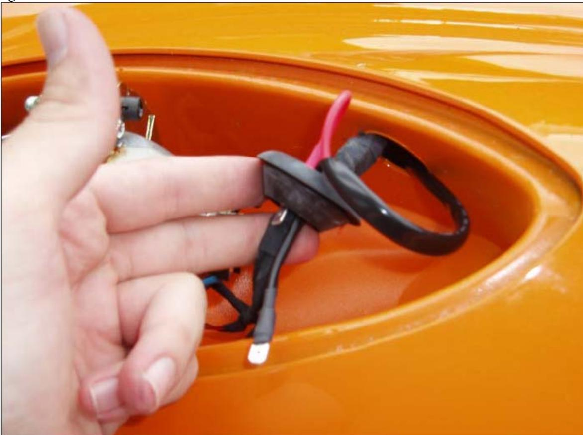
And attach them to the female ends that were attached to the OEM bulb.
