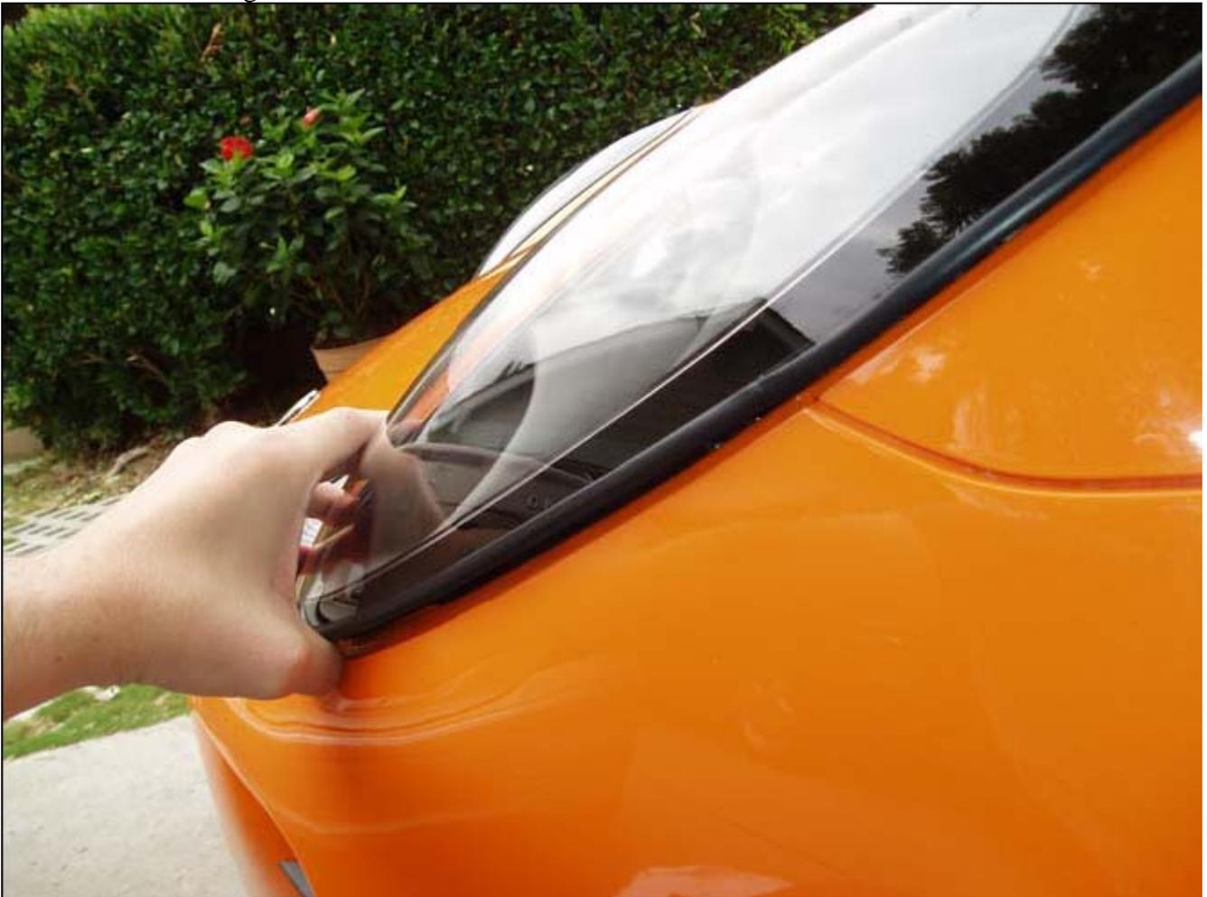
You want to pull forward and up on the lens, because there are some metal clips that the screws, screw into and they want to 'catch' on the light assembly.
