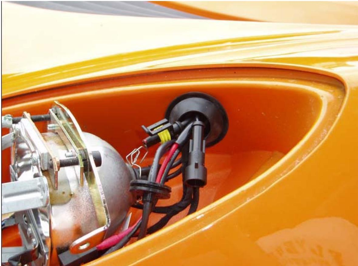
Connect the power-out connectors from the ballast to the wires coming out of the new bulb. And tie that mess up with some fancy colored quick-ties.
