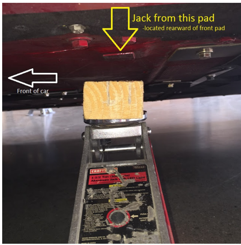
jack from the center pad that is located on the chassis (small red rectangle)
