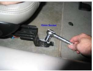
Step 3: Remove Two Front Seat Mounting Nuts
