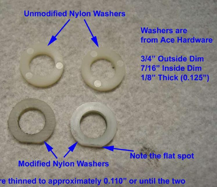
Washers are thinned to approximately 0.110" or until the two washers and one NUT fit without slop in the aluminum block. I used a hobby belt sander, but you can use plain sand paper.
