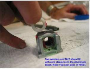
Step 24: Reassemble the Aluminum Block
