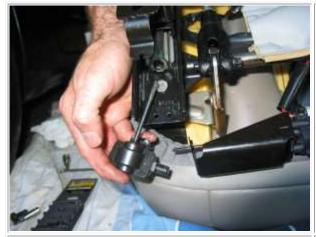
Step 15: Remove Drive Mechanism
