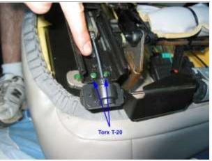
Step 14: Remove Two Torx T-20 Screws Near the Front of the Seat Track
