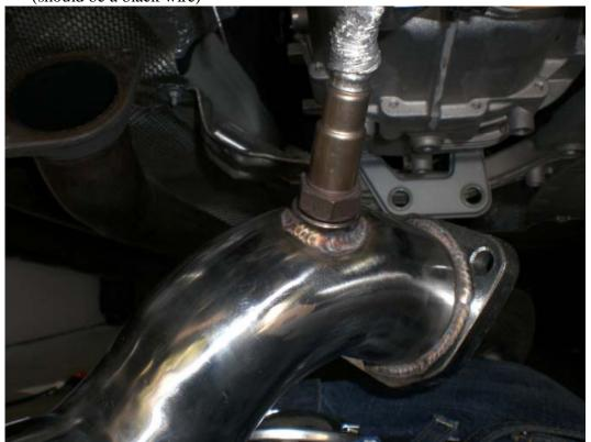
6. Clamp the long pipe up to the turbo and loosely hand tighten the 13mm bolt so there is still play in the pipe.
