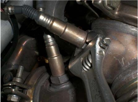
6. Use a 13mm wrench to remove bolts from each turbo clamp. After the removal of the bolts, the clamps should still be tightly in place. Wedge a flathead screwdriver in the clamp opening to break it loose.
