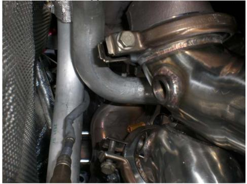
7. Use the gaskets from the stock pipes and the hardware included to bolt the downpipes up to the cat-back using a 13mm socket and wrench.
