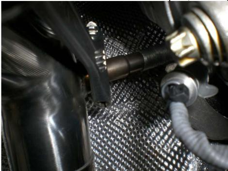
4. Clamp the short pipe up to the turbo and loosely hand tighten the 13mm bolt so there is still play in the pipe.
