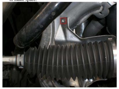
4. Use an E12 Torx driver and 5/8 wrench to remove two bolts securing the steering
