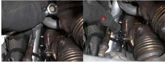
7. Use a 12mm socket to remove four bolts securing the stock downpipes to the cat-back.
