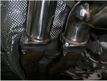
8. Use a 13mm wrench to securely tighten the front turbo clamps. Also, reinstall the front sensors (grey = short pipe, black = long pipe) (if more slack on the wire is needed, release the wires from a clip up above – visible from the top passenger side of the motor)
