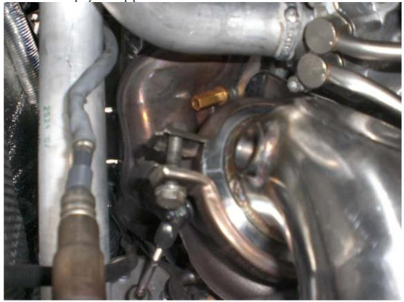
5. Now, for the long pipe. Use a crescent wrench to install the rear sensor in place (should be a black wire)
