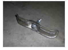
9. Use a 12mm socket and swivel to remove 2 nuts securing the downpipes to a hanger just in front of the rear sensors.
