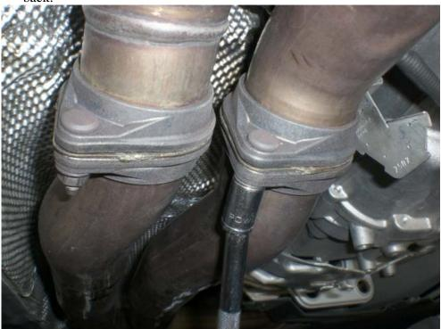
8. Use an E10 torx socket to remove muffler brace
