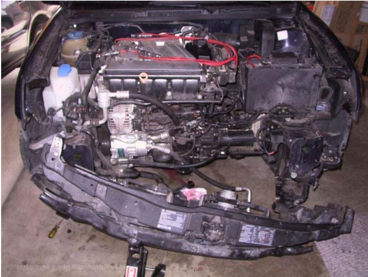
NOTES: Be very careful with how far you move this assembly, as the AC system fittings could be damaged. Also, you can rest the assembly on top of the frame rails when you are not working on the car, and rest the hood on top of this, and it should not come off unless someone yanks on it.
