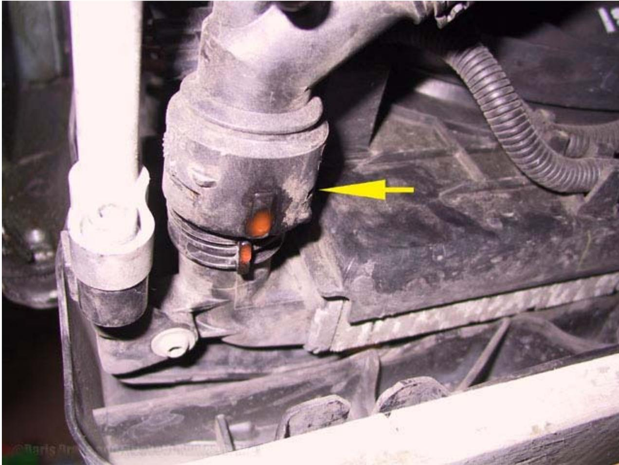
On models with the auxiliary radiator on the passenger side, unclip the return hose leading to the auxiliary radiator.
