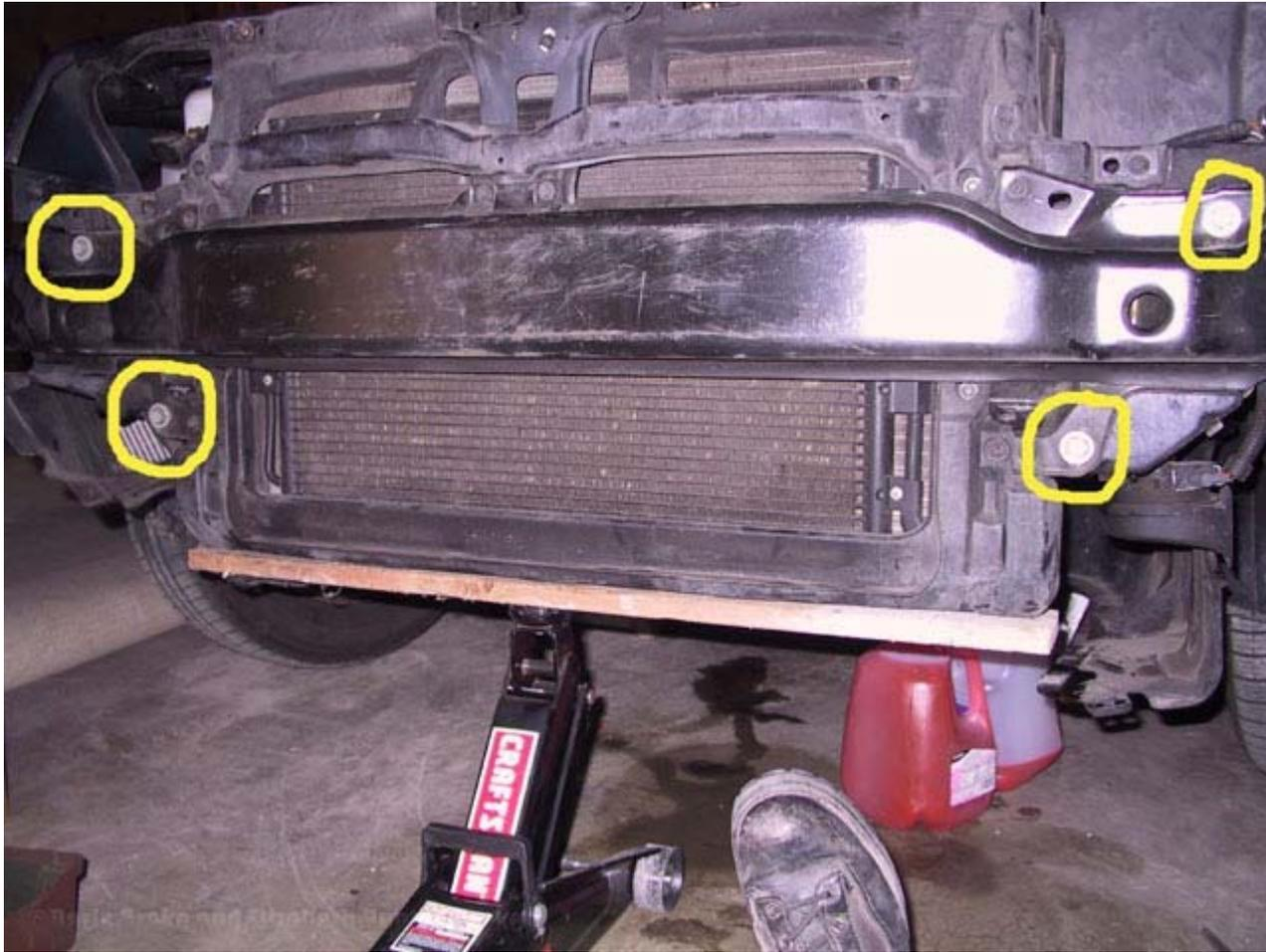
10: Support the lock carrier with a floor jack, and give it a extra centimeter or so extra push upwards to free it. Do not be alarmed, the lock carrier is still held close to the car by the lock cable.
