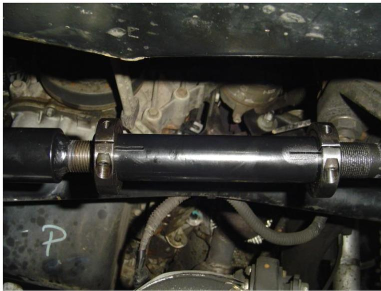
**Quick Adjuster with Shaft Collars Installed**
