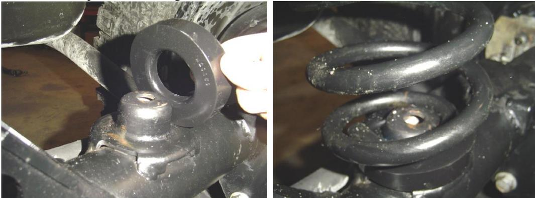
**Note:** *A simple and cost effective way to retain the rear coils to the axle is to use a hose clamp up through the center hole of the spring pad and clamp it around the bottom winding of the coil spring.*
