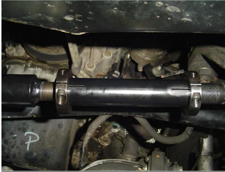
Quick adjuster with shaft collars installed
