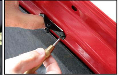
B. Set bracket aside. Using a center punch and a hammer, tap the center of the mark you just made.
