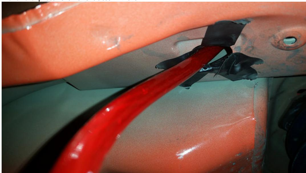
It might not be a bad idea to get some grommets or some other type of insulation material to put around the oval holes to prevent the power cable's insulation from rubbing off due to friction with the sheetmetal (I need to go back and do this).
