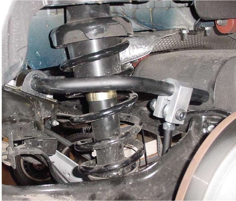
Step 8. Have another person raise the rear subframe while you get the subframe bolt started. Start the inner bolt first. It will appear that the subframe has shifted to the rear of the car, but you will find that the geometry of it will cause it to be pretty close when you raise it back into position. Get all four bolts started first, then tighten them all. There are no slots, so you can't mess up the alignment.
