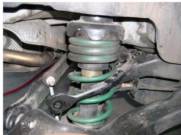
Step 3. Remove one of the rear shock. Start by taking the ABS sensor line and the brake line off of the strut mounts - they just wiggle on and off. Then remove the lower 21mm bolt that holds the strut to the rear hub carrier.
