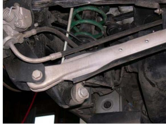
You can see the lower bolt here - it's the one with the triangular plate behind it. After you pull that, take the upper strut 13mm bolts out. There are two. They come out from under the car, so you don't have to even open the rear boot. Once those three bolts are removed, the strut just comes right out.
