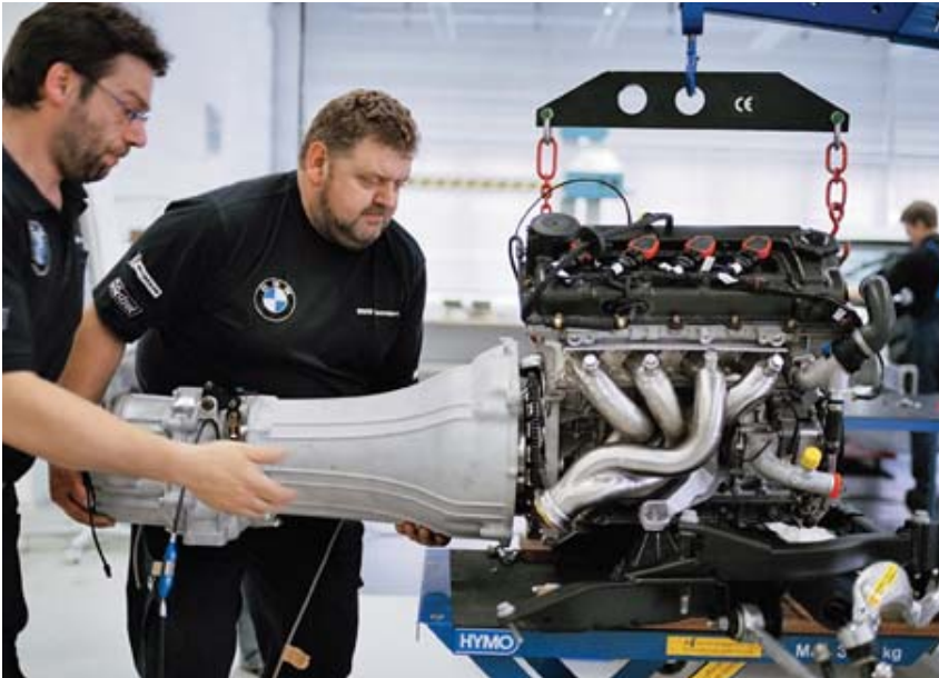
■ BMW Motorsport technicians attach the 5-speed, dog-type racing gearbox to the 320si's P45 2-liter, 275-horsepower engine.
