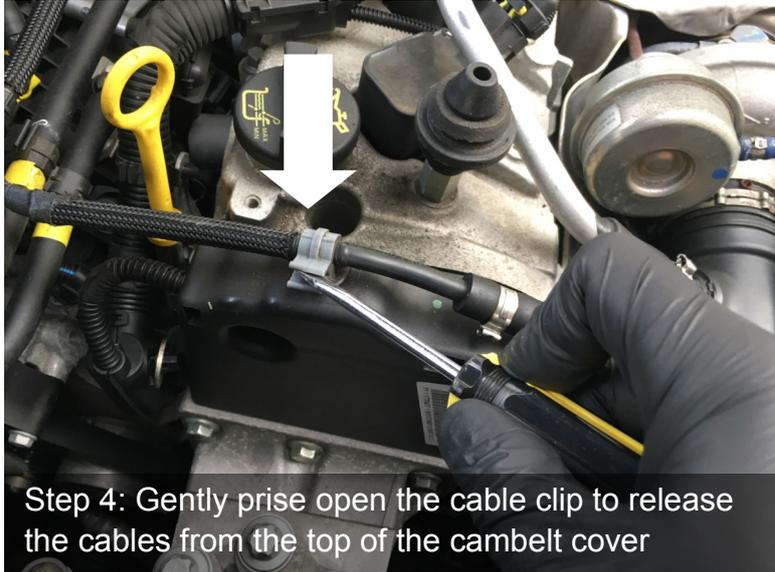
Step 4: Gently prise open the cable clip to release the cables from the top of the cambelt cover
