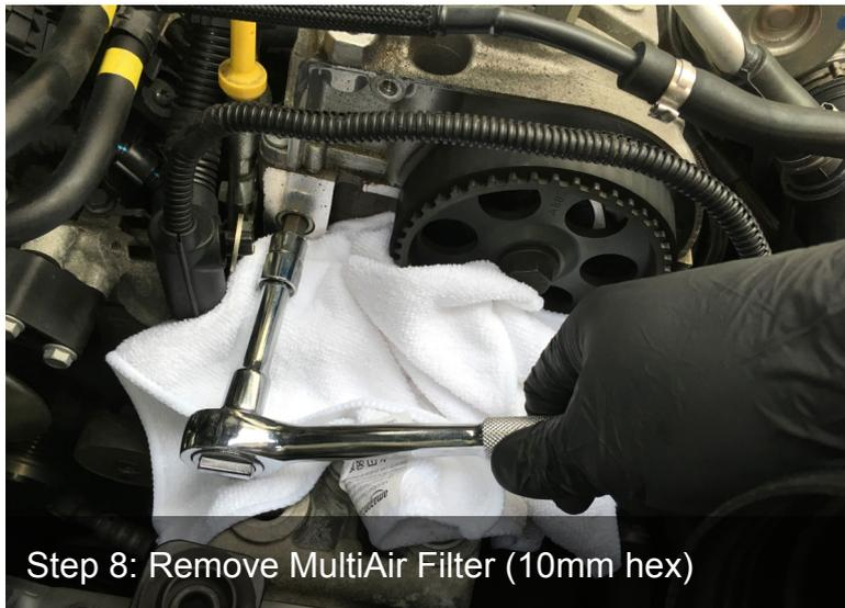
Step 8: Remove MultiAir Filter (10mm hex)
