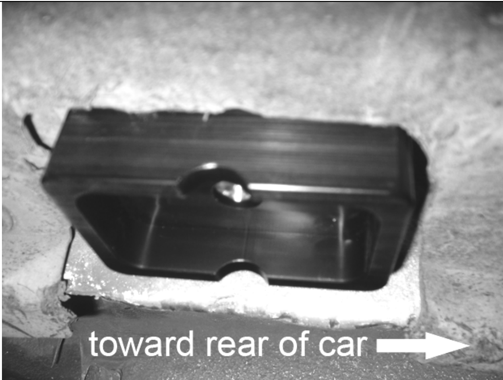
Front jack point installed.
