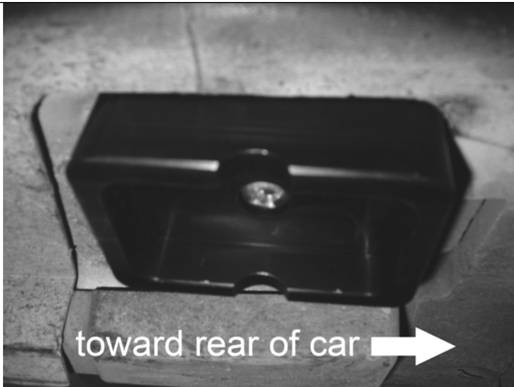
Rear jack point installed.
