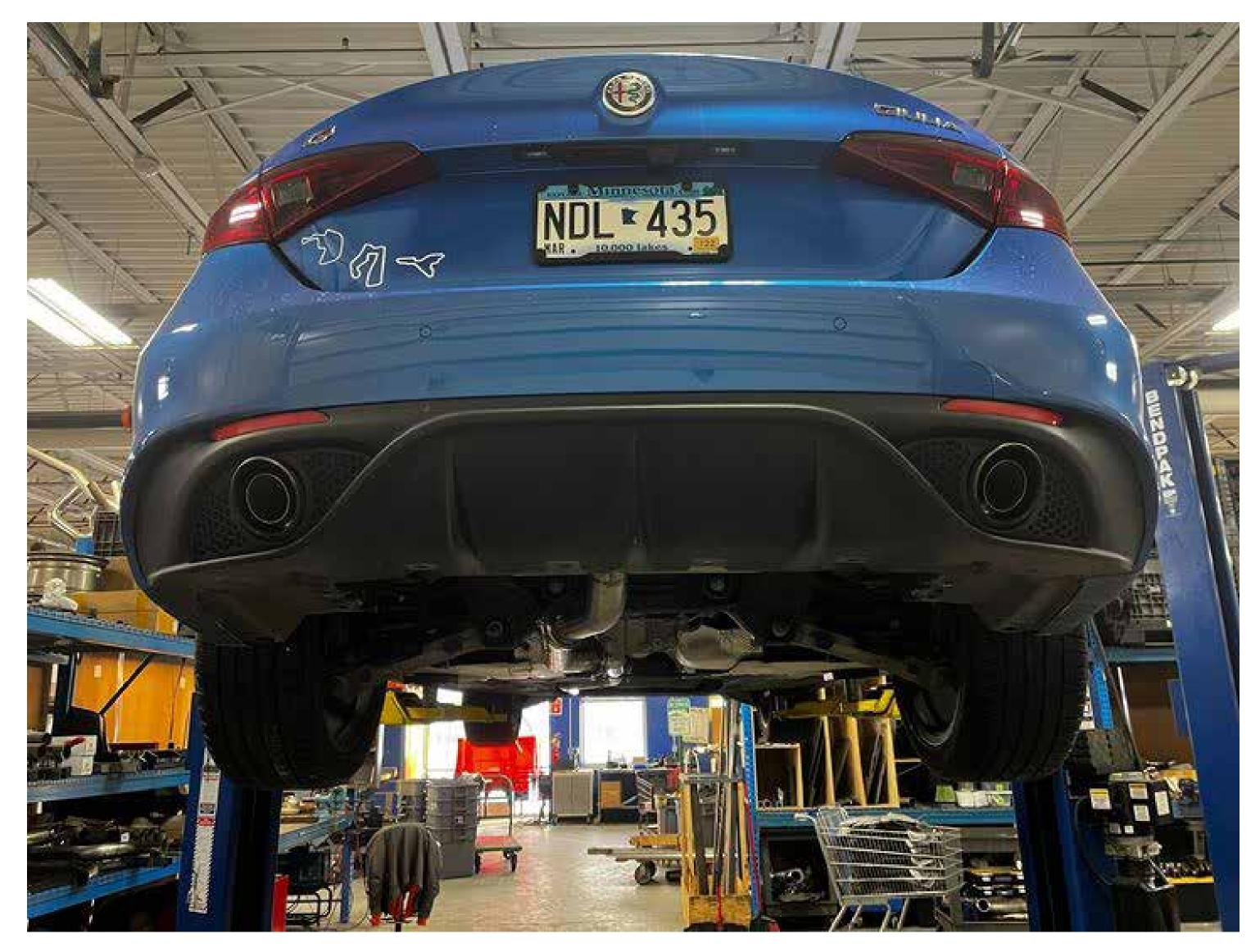
Verify tip placement is center and even on both sides, if not you will need to adjust by loosening the 2 slip clamps and rotating until it fits correctly
