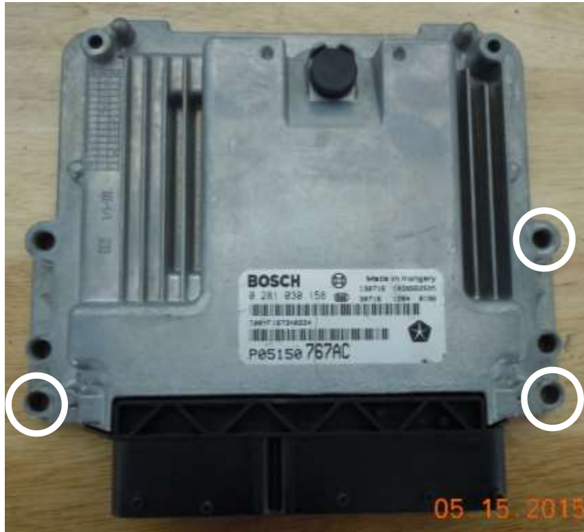
EDC17C79 engine controller for Jeep Grand Cherokee EcoDiesel.
