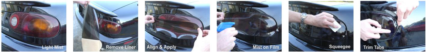
**IMPORTANT: LAMIN-X FILM TEMPERATURES MUST BE GREATER THAN 70 °F (21 °C) FOR PROPER INSTALL!**
