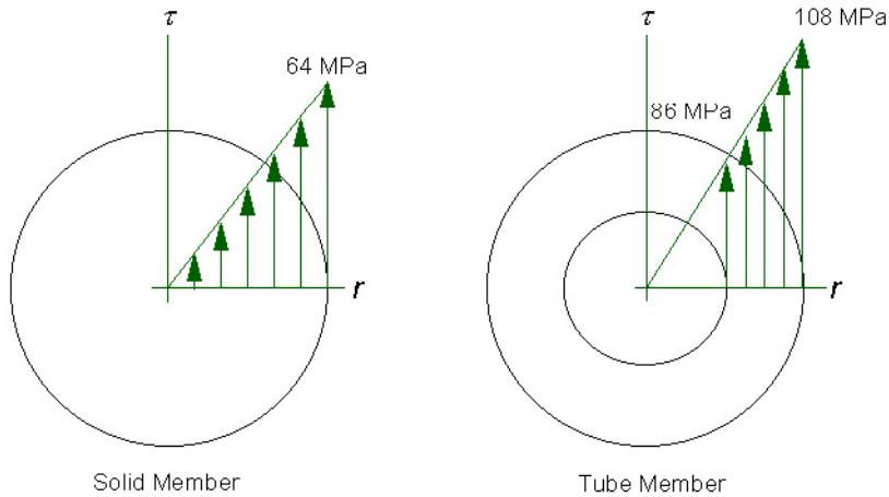
The figure shows graphically how the outer layers of the members carry the most stress. This can make the tube member more susceptible to failure due to surface or wall imperfections and damage.
