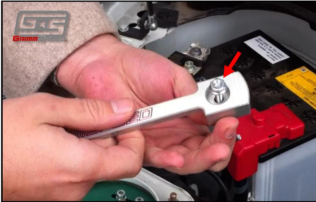
Figure 1: Loosely attach rear j-bolt to the tie down.
