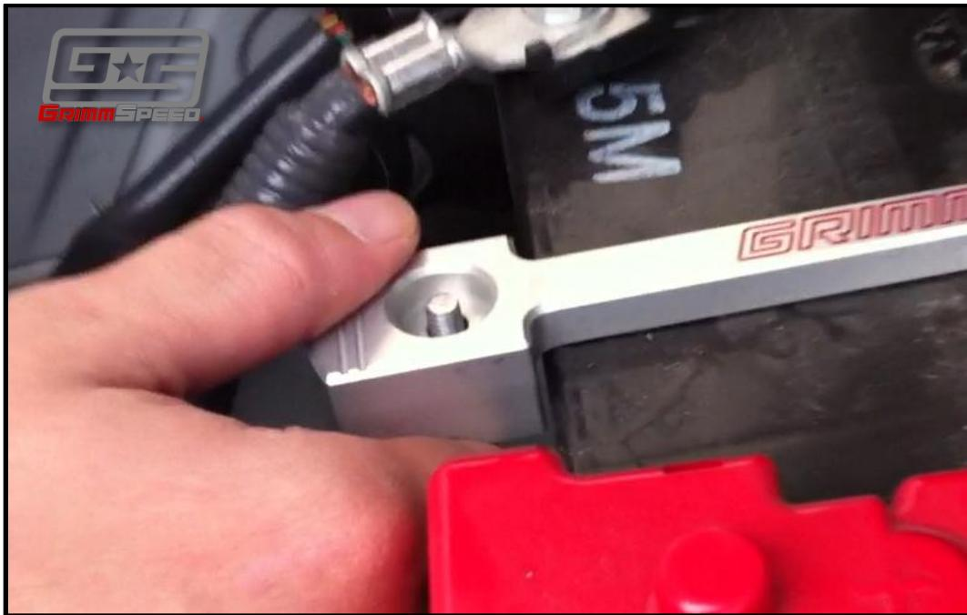
**Figure 3: Hook the front j-bolt.**
