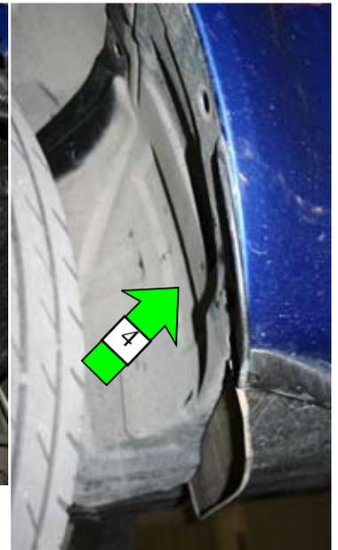
10) Remove the large splash plan (5) mounted between the two fender liner sections. Search around the edges for the different fasteners, they should be pretty easy to find. There are two that are hidden by the fender liners, so be sure to take the liners off first.
