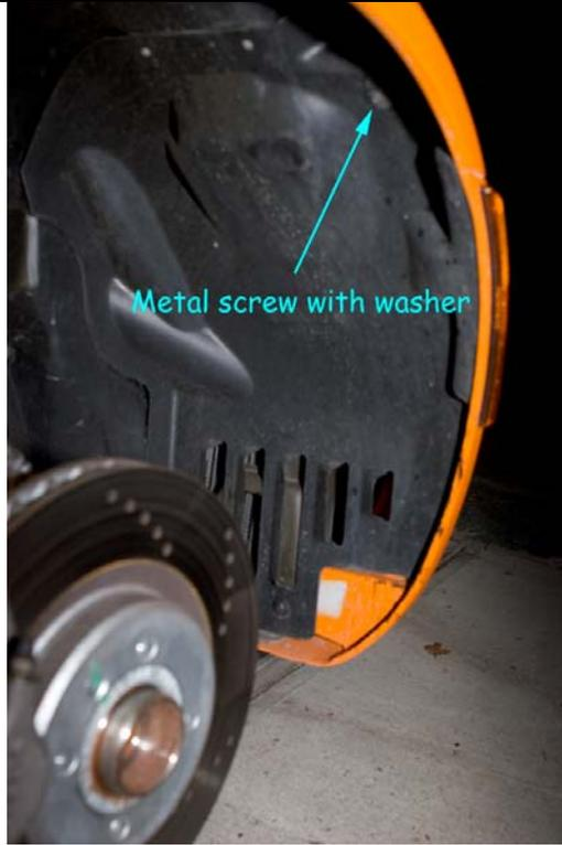
To remove the plastic expanding rivets, use a Phillips screwdriver to extract the screw, but not all the way and then use the exposed screw as a handle to pull the base of the rivet out.
