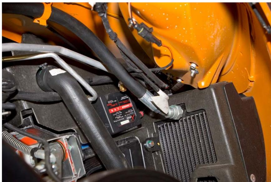
Use a ¼” drill bit to make a hole. While I don’t believe there’s anything behind there, try to check to make sure and don’t push like a monster on the drill. Just apply enough force to let the drill do the work and you’ll break through rather lightly.
