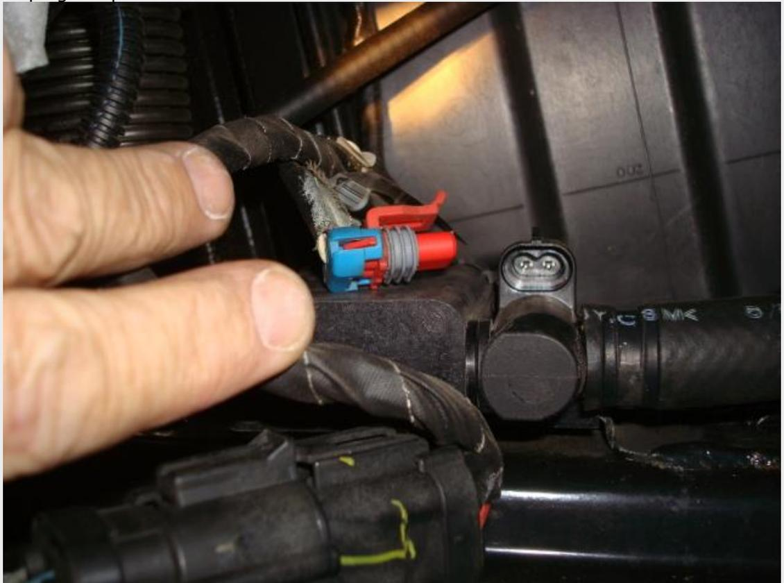
Slide the Vent Solenoid Assy off its bracket. Although it looks like it would slide towards the front of the car it does not. Simply lift the back of the assy high enough for the dog ear to clear the back of the bracket and slide toward the rear of the car. The pic below shows you how it mounts and the dog ear location.
