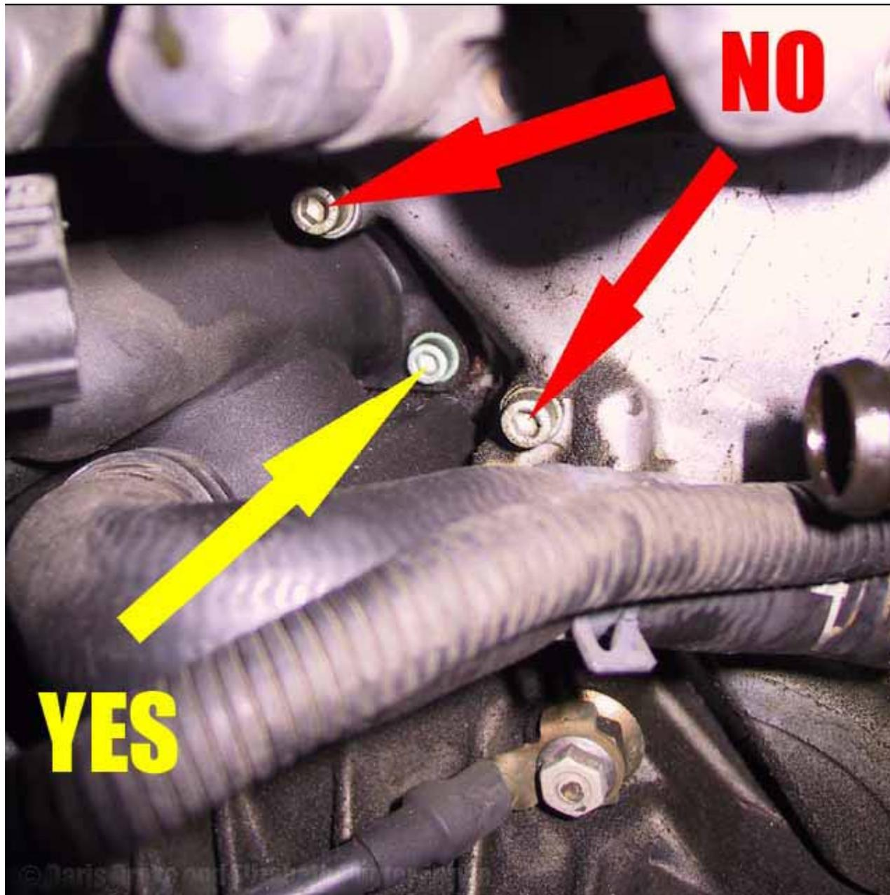
9: Remove the thermostat housing. First break the seal free and then work it out through the front of the vehicle. Set it aside for the next section so we can check sensor condition etc.
