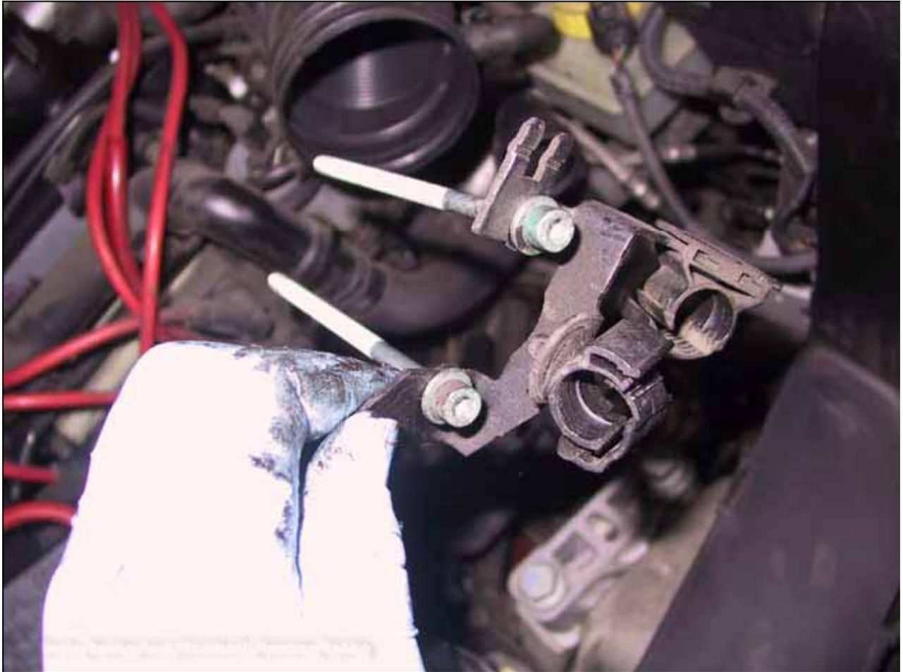
Here is a picture of where this smaller one is located. Be sure you have the right bolt, as the other two pictured are for the timing chain cover.
