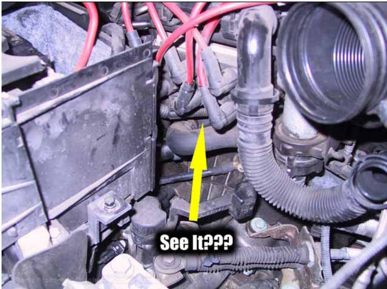
2: Remove the top engine cover (the thing with the chrome Vr6 emblem). This gives you easier access to the coolant and smog pump lines just beneath the coil. To do this first pull the spark plug wires using the tool and pull them from their channels, then remove the six or so T25 Torx screws. Then remove the oil filler cap and pull the cover, and replace the oil filler cap. I would also put the screws for the cover back in their holes just to keep track of them.
