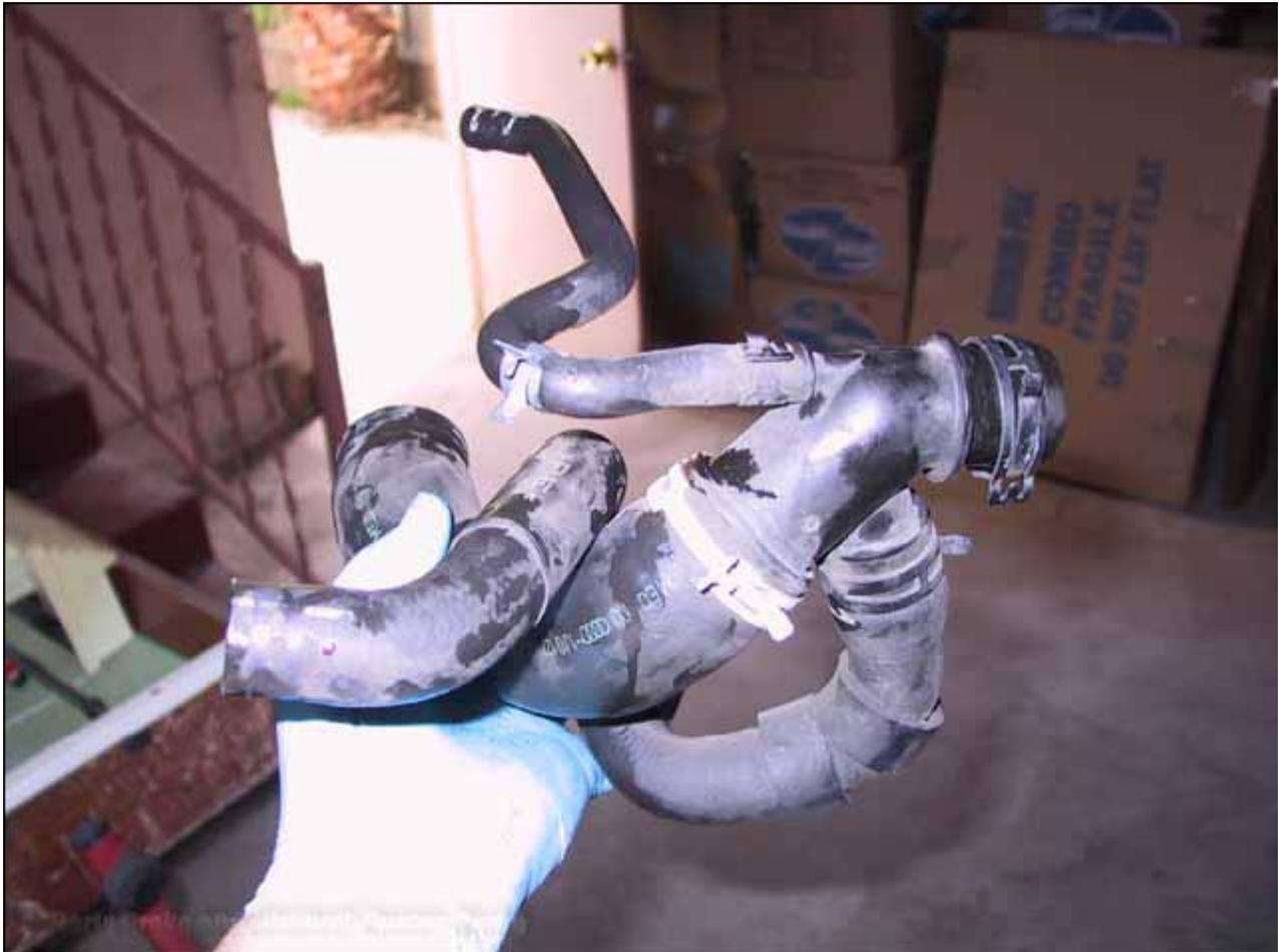
5: Now remove the lower thermostat housing hose. This one is particularly difficult to get at as well. See the yellow arrow in this image:
