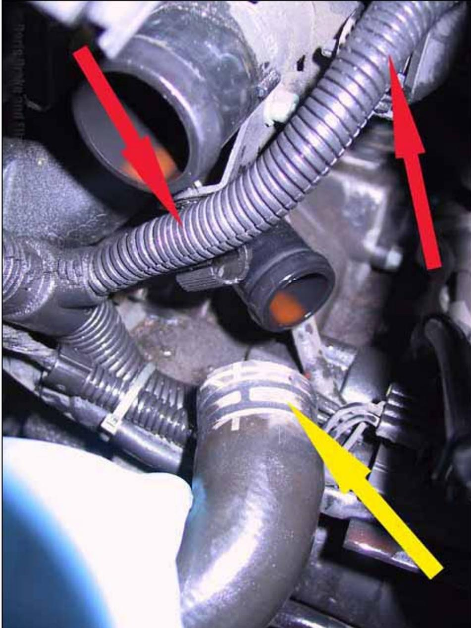
6: Carefully unclip the electrical conduit attached to the bracket on the outside of the thermostat housing. See the image above, the red arrows. Two are shown, there are three total. Now we will move to the back part of the housing.
