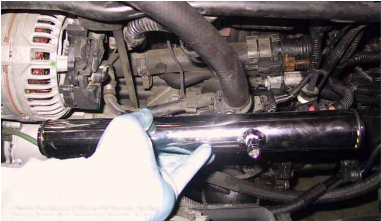
15: Drain the crack pipe. This one is messy. The drain has to be accessed from underneath the car, and is just next to the block where the water pump housing fits. The stock pipe will need a flathead screwdriver and a turn or two, then it pops off. **WEAR EYE PROTECTION!!!**
