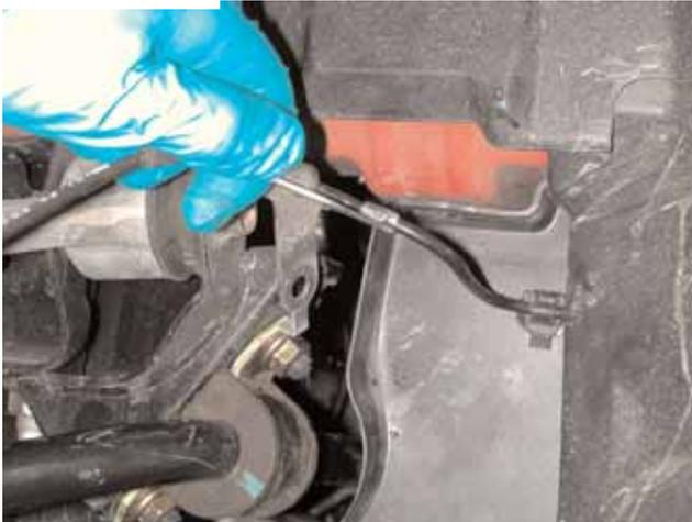
7. Using a 5mm Allen wrench and a 14mm combination wrench, remove the nuts attaching the top of the anti-sway bar end links to the anti-sway bar. Remove the end links from the anti-sway bar. Using a 14mm combination wrench, remove the nuts that secure the anti-sway bar brackets to the vehicle. Remove the brackets and the bushings from the bar. Illustration 7.
