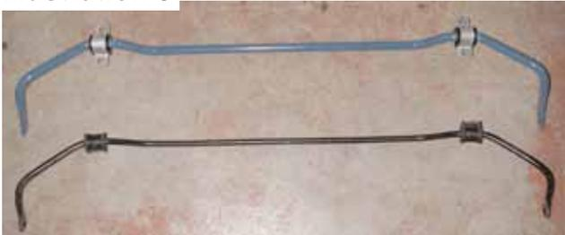
4. Install the new bar in the vehicle as the factory bar was. Reattach the end links to the bar before tightening the bracket nuts. You may want to start by installing the end links through the forward most holes in the bar as this is the softer setting. Torque the four nuts attaching the brackets to the vehicle to 15 ft lbs. and then the end link nuts to 32 ft lbs. Illustration 4.
