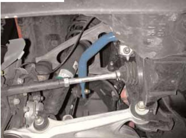
11. Reinstall the ABS wheel speed sensor wire brackets and the splash shield bolts to the vehicle. Reinstall the wheels and snug the lug nuts. Remove the jack and jack stands. Torque the lug nuts to 80 ft lbs. Enjoy your new Anti-sway bars!
