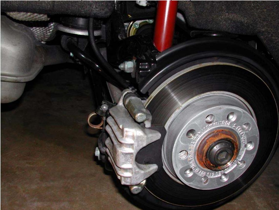
10. Re-attach wheel. Be sure to use the star pattern, and if you have a safety bolt be sure to put that one directly opposite of the valve stem. Also tighten that one last. Torque to 92 lbs/ft.
