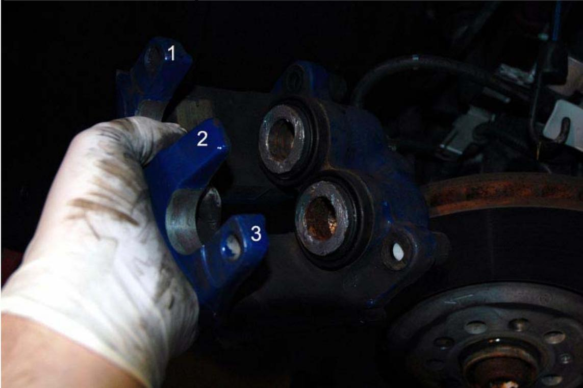
Pop the wear sensor into the new pad, snap the pad into the two pistons, put the front pad in the mounting bracket, and screw back in the caliper screws and put back the front retaining clip – you're all set! I did not have to push back the pistons as I only have 4900 miles and the pads weren't very worn. If you did have to push back the pistons, I would just stick a big set of pliers in-between the pads and expand them, thus pushing back the pistons.
