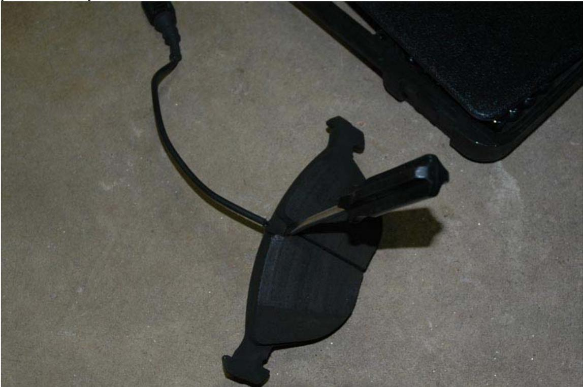
Get a flat head screw driver, fit it behind the sensor and push it out. If you are careful, the sleeve that the sensor sits in will remove with the sensor. You'll see what I mean when you do it.
