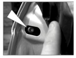
Slide out the exisitng door lock mechanism. (Once the scew is removed, the mechanism will come out with ease.)
