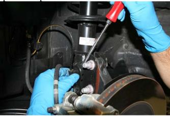
3) Remove the 12mm bolt that attaches the brake line to the front strut and pull the brake line out of the way.
