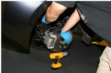
5) Remove center top nut and remove top mount, dust boot, bump stop, and spring from shock. Pull up on the top mount as you are loosening the top nut to keep pressure on the nut and prevent the shaft from spinning. Use extreme caution: the top mount will pop off with force. Eye/face protection is recommended.
