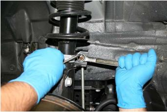
5) Remove two lower 19mm clevis nuts/bolts.
