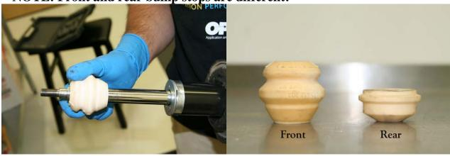
12) Compress RCE spring using spring compressors and place onto strut, making sure that it is oriented correctly in the spring seat.
