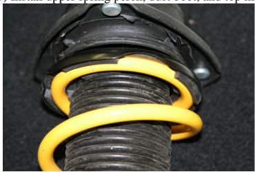
14) Install top nut and torque to 41 ft-lb.
