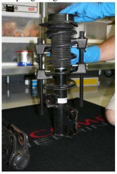
9) Remove 17mm center top nut and pull top mount, dust boot, upper spring perch, and spring off of strut.
