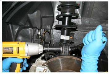
6) Remove three upper 12mm nuts that fasten strut top mounts to chassis.
