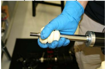
11) Install RCE bump stop onto shaft.
