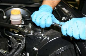
7) Remove strut/spring assembly from vehicle.
