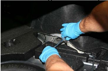
4) Push down on swingarm and remove shock from vehicle.
