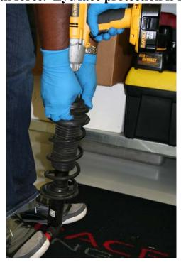
6) Slide RCE bump stop into groove at the top of RCE dust boot with the flat side facing up. Install RCE bump stop/dust boot onto shaft.
