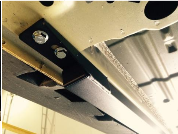
Figure 2: Passenger Side Jacking Rail
