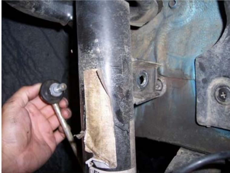
**5. Detach Strut from Spindle**
