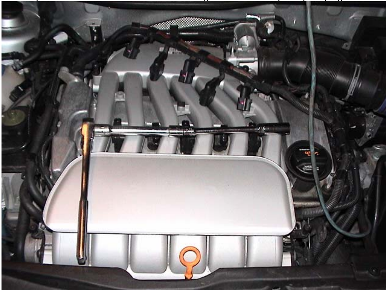
9. Now you will need a wrench and an uber long extension with your spark plug socket.
