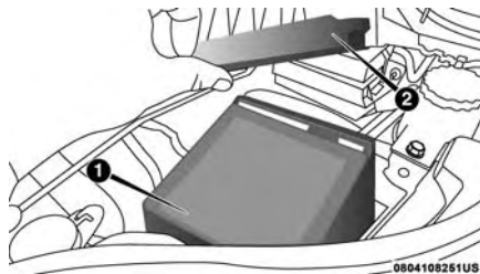
Open Air Cleaner Filter Assembly
