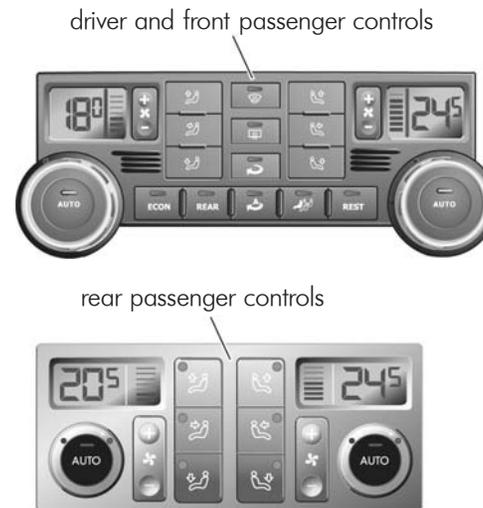
As for the 4-zone CLIMAtronic's indirect ventilation, it is simply unmatched. With it, the air flows smoothly over a broad area of the Touareg's upper dash panel. The air vents in the B-pillars also contribute to smooth air flow by keeping the side windows free of moisture, and a sensor ensures that the humidity remains within a pleasant range.
