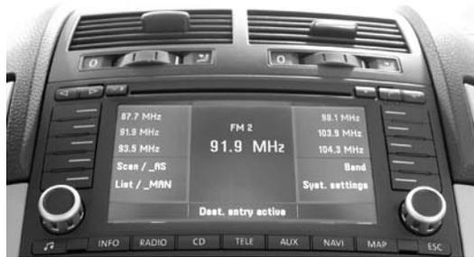
this unit, the stereo controls are integrated within the Navigation display. One important note for customers is if the Navigation CD is being used in the vehicle, then they will be unable to play music CDs. Suggest the optional 6-disc CD changer to customers for whom music CDs and Navigation are especially important.
